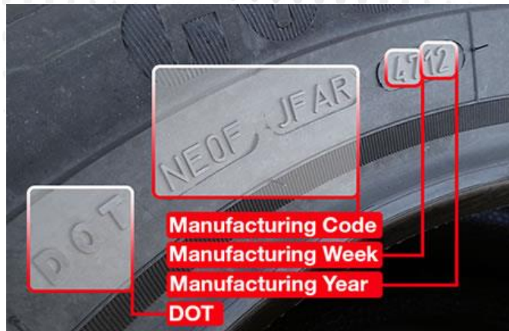
Fig; 2 – This tyre was produced in calendar week 47 of 2012
